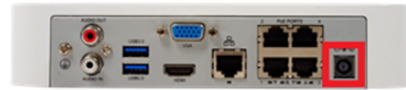
One end of the NVR Power supply to the back of the NVR and the other end (prong) to a wall power outlet
